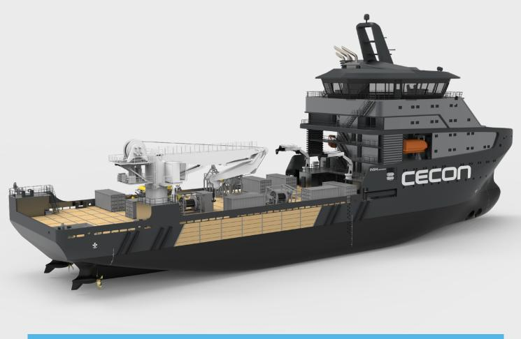
The new built Cecon TBN is a groundbreaking state-of-the-art cable installation vessel which will be delivered from Sefine Shipyard in Turkey Q1 2025. With a battery package for hybrid energy storage and dual fuel generators for Methanol fuel, the vessel has a significant reduction in harmful emissions compared to existing conventional tonnage.
